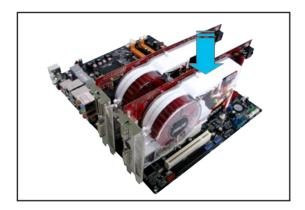
Connect an auxiliary power source from the power supply to the graphics cards.
