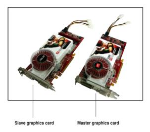
Insert the CrossFire™ Edition (Master) graphics card into the PCI Express x16 orange slot. Make sure that the card is properly seated on the slot.
