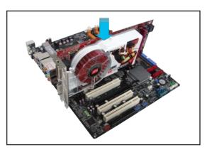
3. Insert the CrossFire™-ready (Slave) graphics card into the PCI Express x16 black slot. Make sure that the card is properly seated on the slot.
