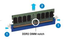
2. Remove the DIMM from the socket.
