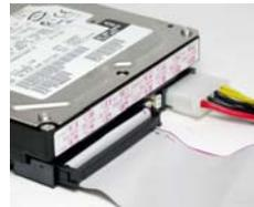
IDE devices enclose jumpers or switches used to set the IDE device as MASTER or SLAVE. Refer to the IDE device user's manual. Installing two IDE devices on one cable, ensure that one device is set to MASTER and the other device is set to SLAVE. The documentation of your IDE device explains how to do this.
