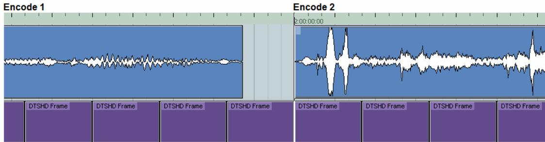
Figure 10-9 Join: Gap in Audio
