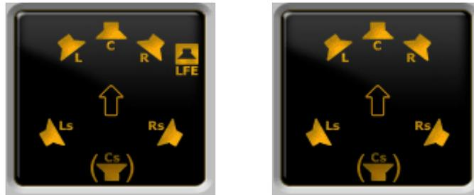
Figure 7-19 6.0 and 6.1 ES Matrix Phantom Speaker Layout
