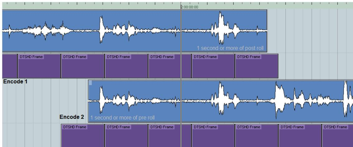
Figure 10-5 Join Overlap Diagram (not to scale)
