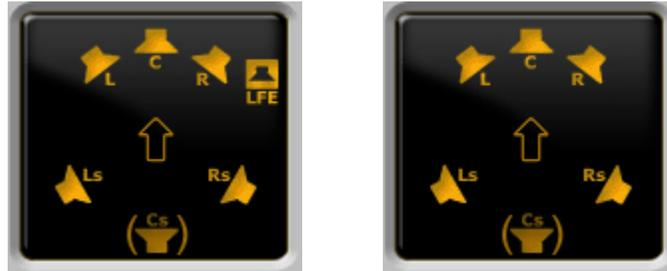
Figure 7-17 6.0 and 6.1 Matrix Phantom Speaker Layout
