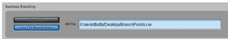
If the Seamless Branching feature will be utilized on a Blu-ray Disc, all encodings created for that disc should use a Seamless Branching mode: *Single Clip* or *Use CSV Branch Points*.
