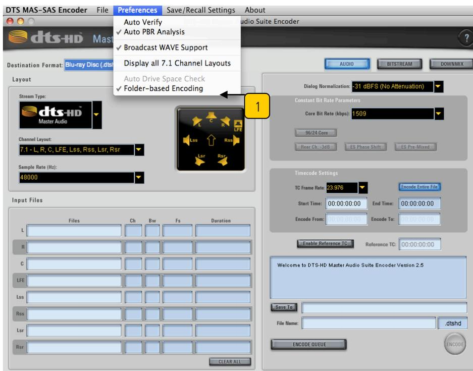
2. Select appropriate *Destination Format*, *Stream Type*, *Channel Layout*, and *Sample Rate*. These settings will apply to all encodes in the batch.
